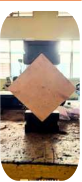
Diagonal shear test setup for masonry wall
